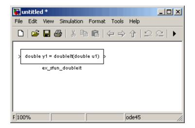
The following Simulink model demonstrates that the C MEX S-function produced by the Legacy Code Tool behaves like the C function doubleIt. In particular, the S-Function block named ex\_sfun\_doubleit returns the value of its floating-point input multiplied by two.
