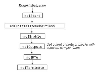
If the S-function resides in a conditionally executed subsystem, it is possible for the generated code to interleave calls to mdlInitializeConditions and mdlStart. Consider the following Simulink model sfcndemo\_enablesub.mdl.
