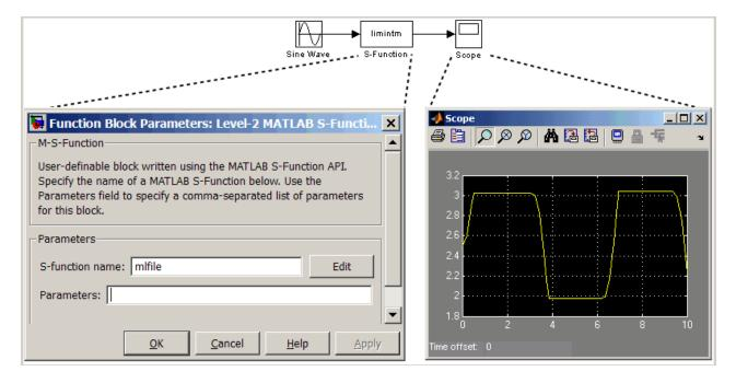
The model in this example incorporates the sample S-function msfcn\_limintm.m.
