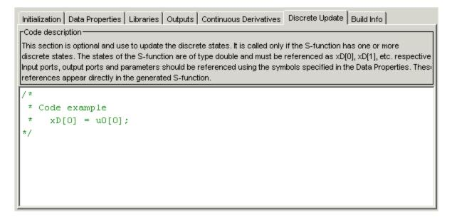
Enter code to compute the values of the discrete states in the **Code for the mdlUpdate function** field on this pane. When generating code, the S-Function Builder takes the code in this pane and inserts it in a wrapper function of the form
